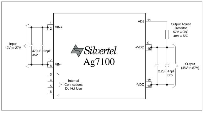
Figure 3: Typical System Diagram
