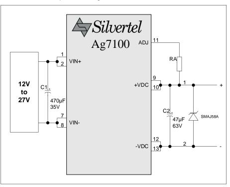
Figure 11: Ag7100 Output Protection
