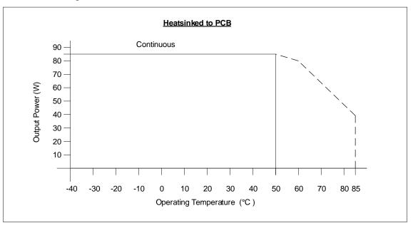
Figure 13: Operating Temperature (Thermally connected to PCB)
