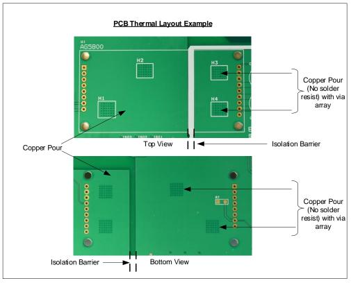
Figure 14: Suggested PCB Thermal Layout
