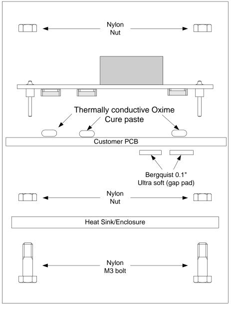
Figure 16: Suggested Heat Sink Assembly
