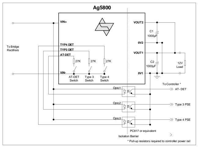
Figure 5: Physical Layer Detect Configuration
