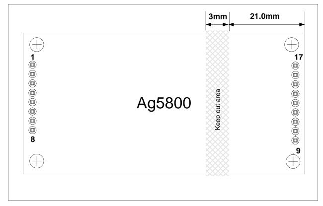
Figure 17 shows the position of the isolation barrier on the bottom of the Ag5800.
