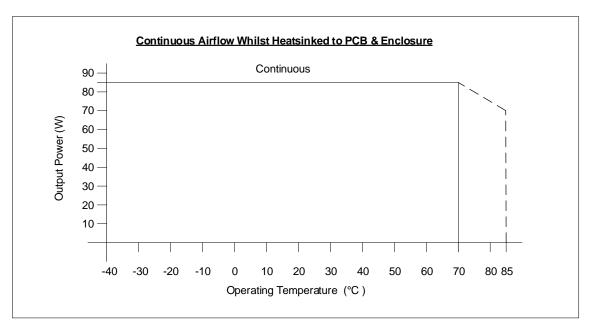
Figure 11: Operating Temperature
