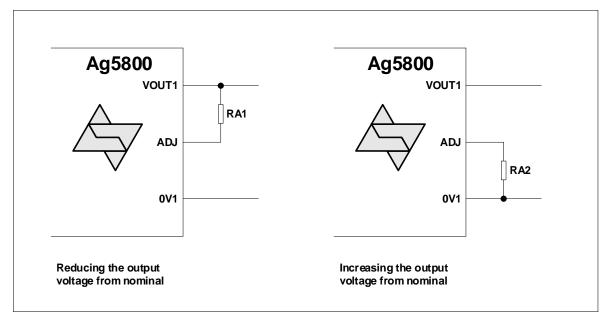
Figure 7: Output Adjustment
