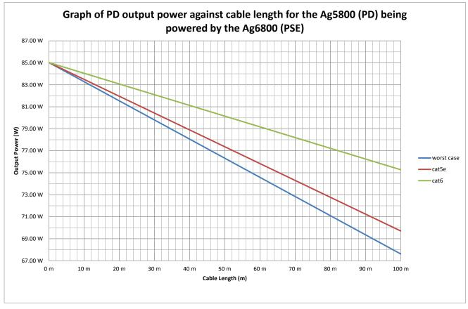
Note: This was calculated using typical cable resistances and with schottky bridge rectifiers part number: SS36 (Vf of 0.5V at the operating current) - Ag6800 supply voltage of 55V.
