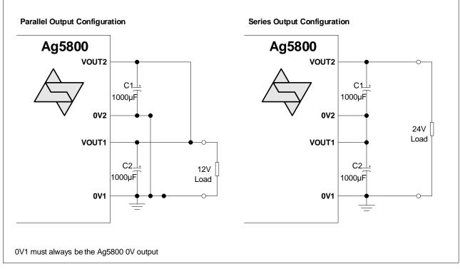
Figure 6: Output Configurations
