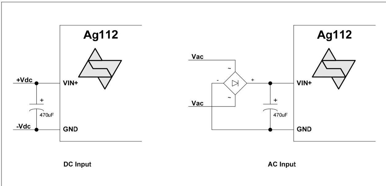
**Figure 4: Input Connections – DC or AC Input**
