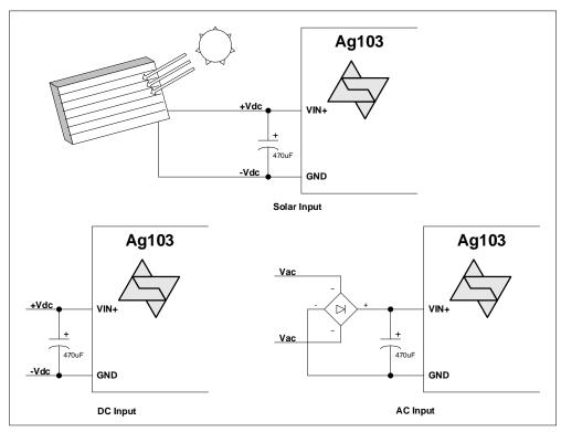
Figure 4: Input Connections – Solar, DC or AC Input
