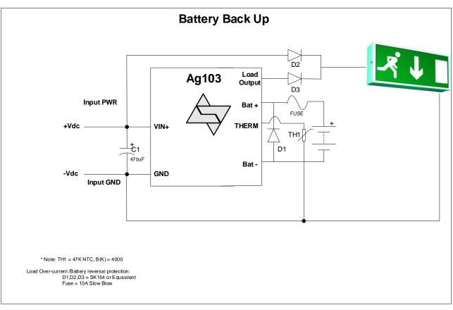
Figure 10: Typical Application - Battery Back Up
