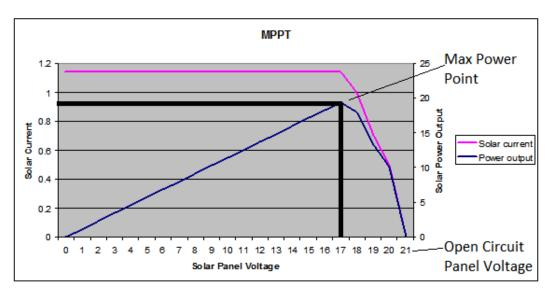
Figure 11 below shows an example of the Maximum Power Point of a 20W panel.
