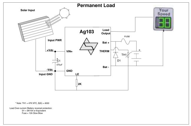
Figure 9: Typical Application - Permanent Load
