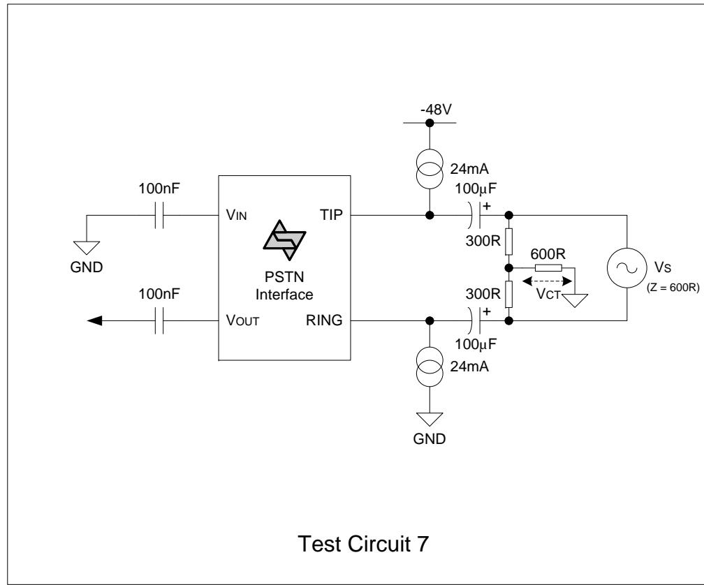
$$\text{Metallic to Longitudinal Balance} = 20 \log(2V_{CT} / V_{T-R})$$
