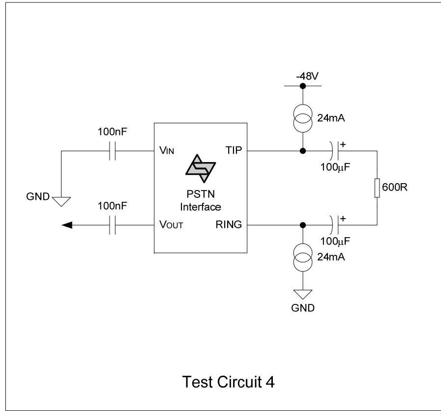
$4W \text{ Noise} = 20 \log(V_{T-R} / 0.775)$  NOTE:  $V_{T-R}$  with a Cmess Filter
