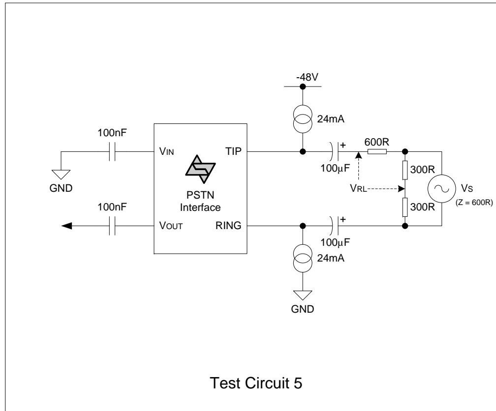
$$\text{Return Loss} = 20 \log(2V_{RL} / V_S)$$
