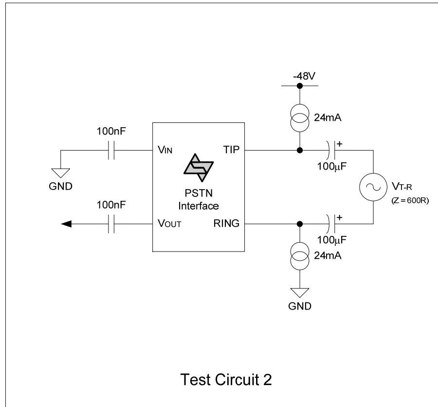
$$\text{Transmit Gain} = 20 \log(V_{\text{OUT}} / V_{\text{T-R}})$$
