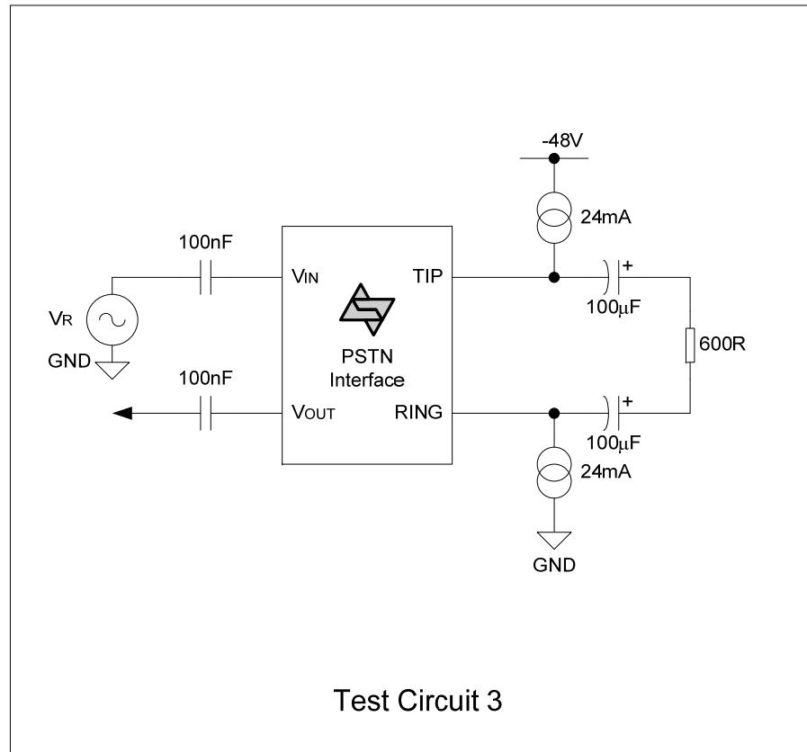
$$\text{Receive Gain} = 20 \log(V_{T-R} / V_{IN})$$
