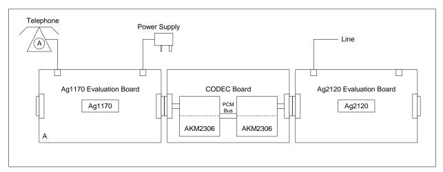
Figure 4: Connecting an Ag1170, Ag2120 and CODEC Boards
