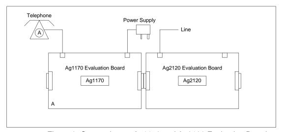
Figure 3: Connecting an Ag1170 and Ag2120 Evaluation Boards
