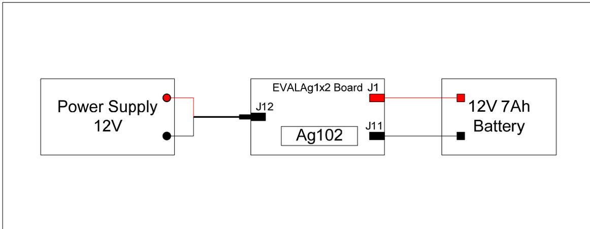
Figure 4: Example set-up
